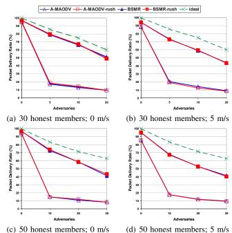
Fig. 7: Black hole attack and flood rushing combined with black hole: **Strategic placement (JOIN)**
