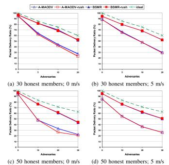
Fig. 6: Black hole attack and flood rushing combined with black hole: **Random placement (JOIN)**
